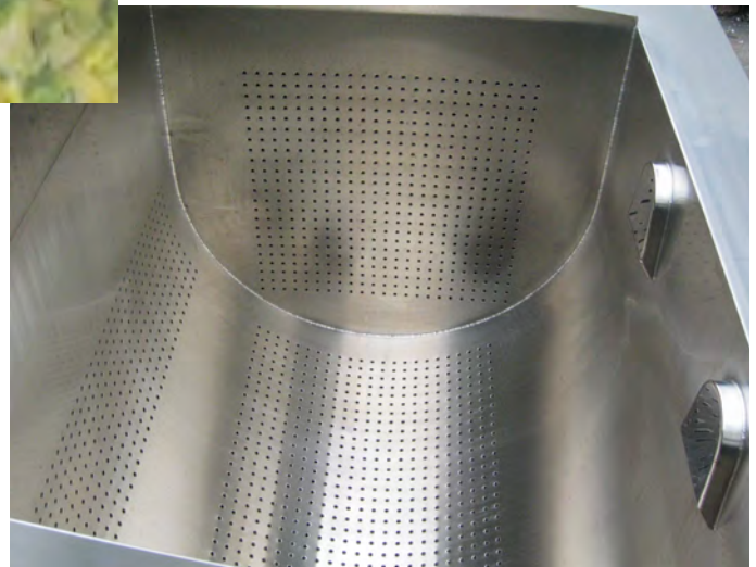
Perforated wash basket with agitation jets
